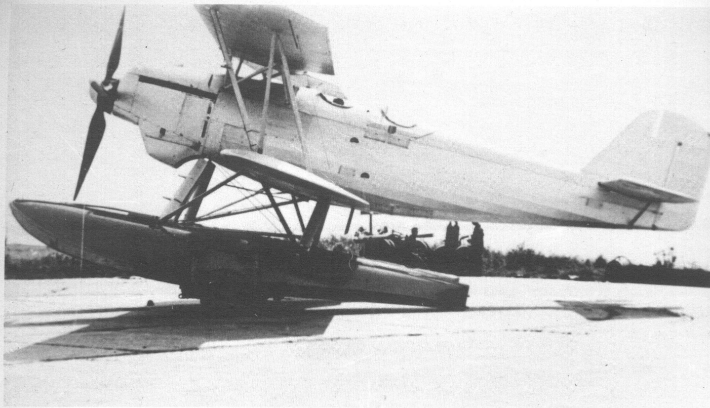
Two photos of the He 60a, which differed from the later versions in a number of respects. Its most noticeable feature is the four-blade propeller. Another is the use of a single strut to brace the horizontal stabilizer instead of the N-strut which was introduced by the second prototype.
