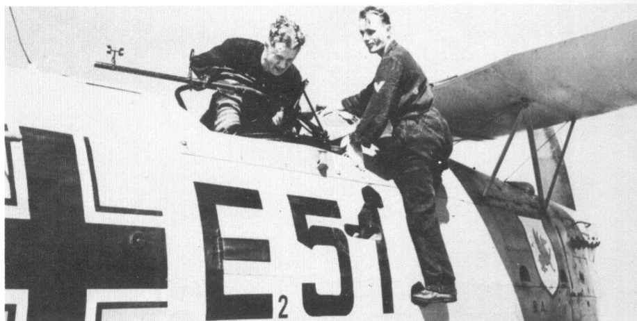
Close-up of an He 60 C with MG 15 machine-gun on a circular-track mount.
