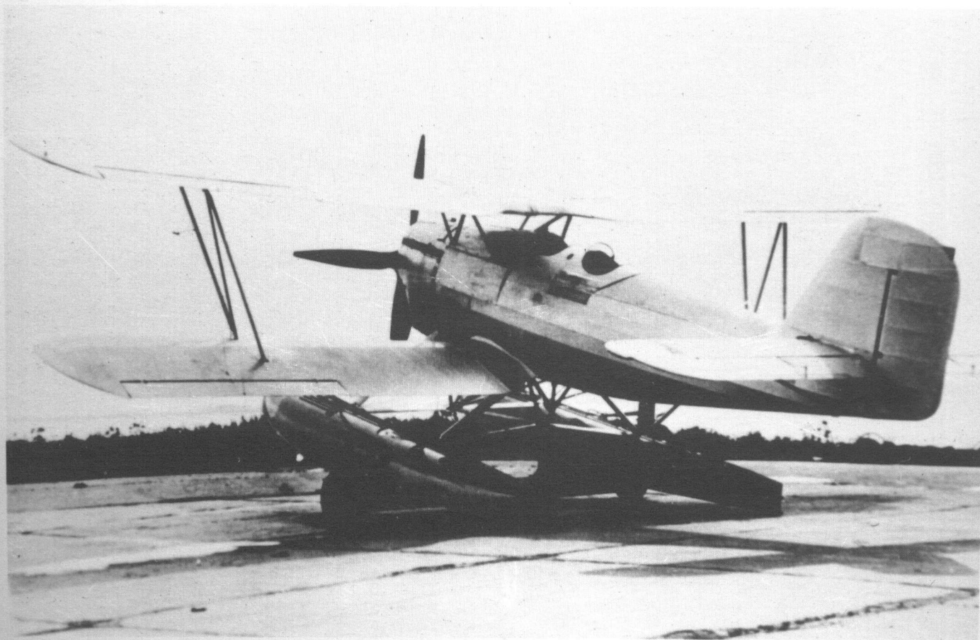
Two photos of the He 60a, which differed from the later versions in a number of respects. Its most noticeable feature is the four-blade propeller. Another is the use of a single strut to brace the horizontal stabilizer instead of the N-strut which was introduced by the second prototype.
